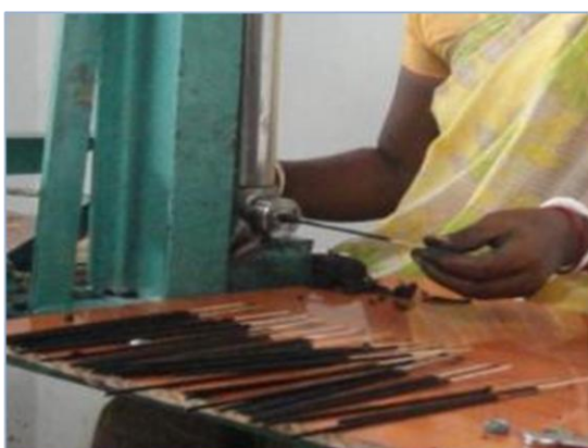
Mechanized Rolling of Agarbatti
