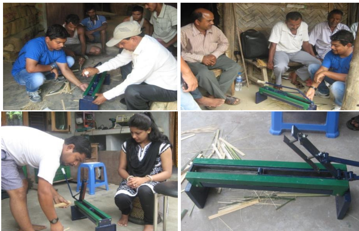
Low cost machine of slicing cum stick making under the innovation drive by Tripura Bamboo Mission
